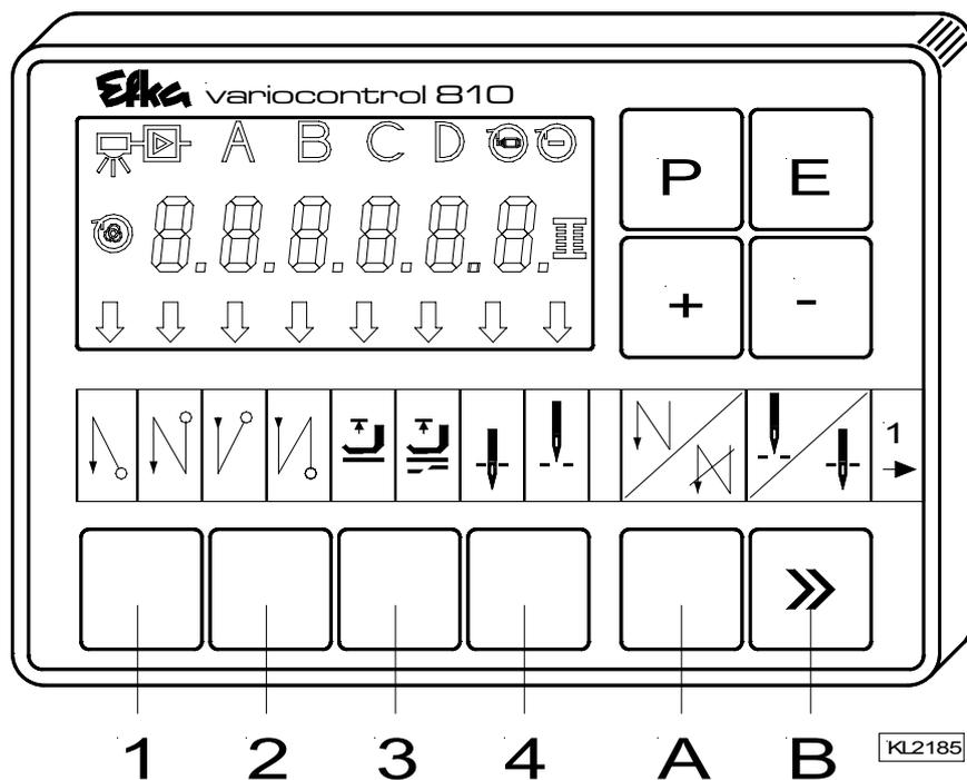
The V810 control panel is supplied with slide-in strip **no. 1** above the keys. For different functions the strip can be replaced with another one supplied with the control panel. Set parameter **291** in this case. See also **V810 / V820** instruction manual!
