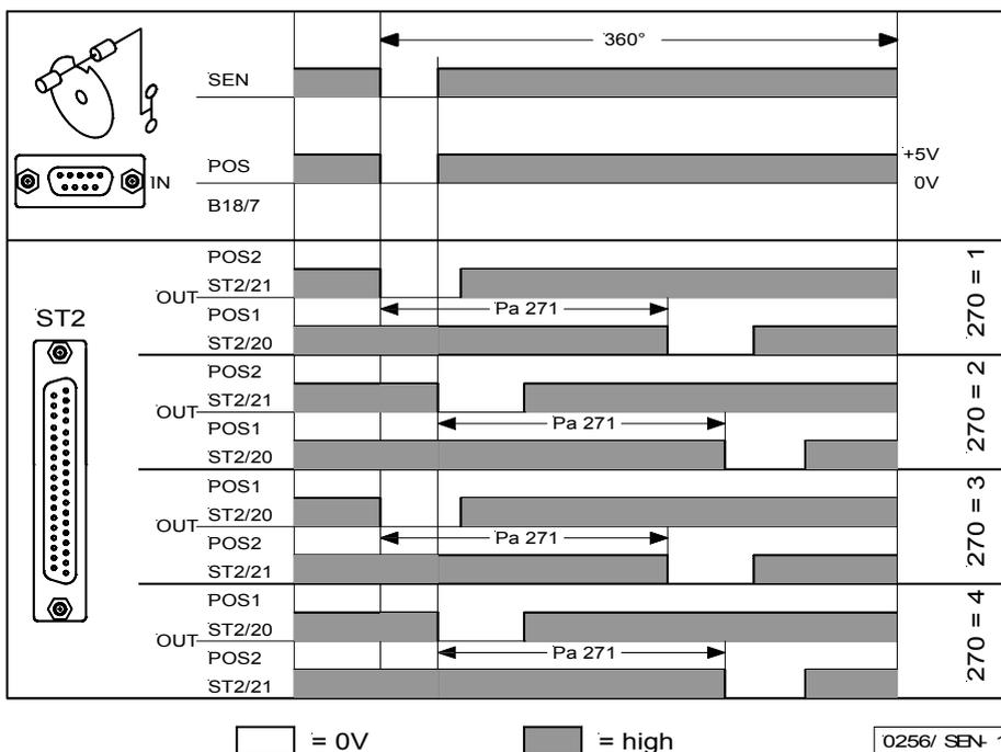
Connection of a sensor (N.C. function) e. g. light barrier or proximity switch to socket B18/7.
