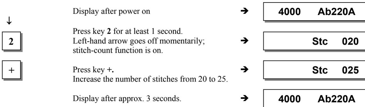
**These values are saved when you start sewing. They remain in effect even after turning the machine off!**
