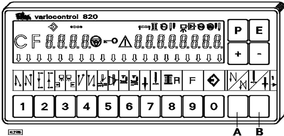
The V820 control panel is supplied with slide-in strip **no. 1** above the keys. For different functions the strip can be replaced with another one supplied with the control panel. Set parameter **292** in this case. See also **V810 / V820** instruction manual!
