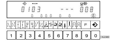
Display of seam 03 after correct function input
