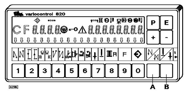
The V820 control panel is supplied with slide-in strip **no. 1** above the keys. For different functions the strip can be replaced with another one supplied with the control panel. Set parameter **292** in this case. See also **V810** / **V820** instruction manual!
