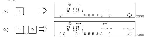
■ Enable all desired functions of the actual seam. as for ex. light barrier, by pressing keys 1...9.
