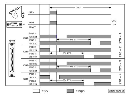
OUT (position window) = npn transistor (emitter to 0V) is conductive. The width of position window cannot be adjusted.
