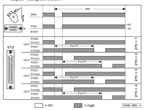
Connection of a sensor (N.C. function) e. g. light barrier or proximity switch to socket B18/7. The following settings are possible using parameter 270:
