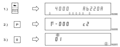
• Activate programming of seams TEACH IN using key 0 / Display of pattern number. Determine new pattern numbers using keys 0...9. Select the next available pattern number using key +.
