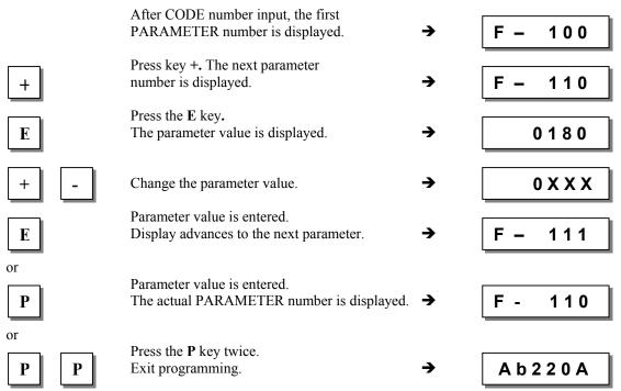
These values are saved when you start sewing. They remain in effect even after turning the machine off. Using parameter 401 is another possibility for immediate storage without having to start sewing.
