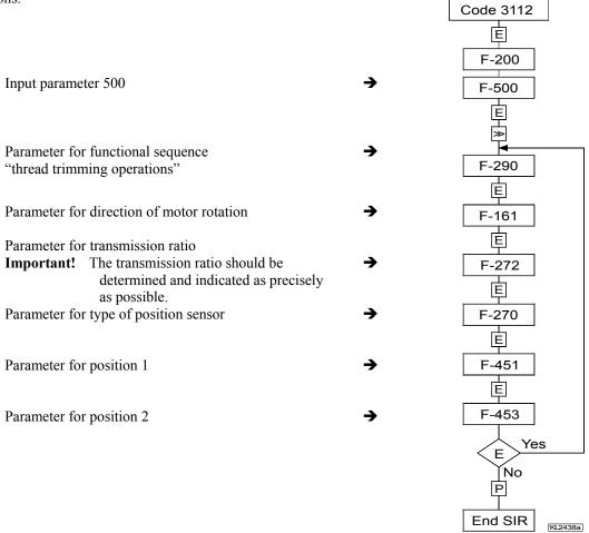
The values can be varied by pressing keys +/-. When the parameter is displayed on the V810 control panel, press the E key once more for the value to be displayed.
