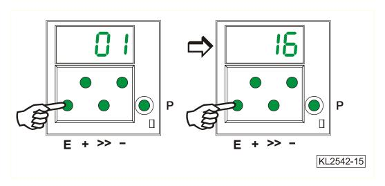
The routine is repeated by pressing the  $\bf E$  key again. Exit the routine after pressing the  $\bf P$  key once. The next parameter number is displayed. Exit programming after pressing the  $\bf P$  key. The drive is again ready for sewing.
