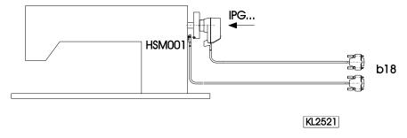
Representation and installation of a HSM001 Hall sensor module  $\underline{or}$  IPG... pulse encoder together with a LSM002 light barrier module by means of adapter cord no. 1113229
