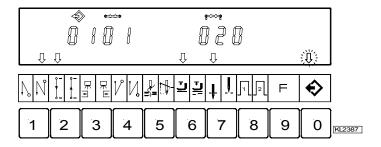
Display of seam 01 after correct function input
