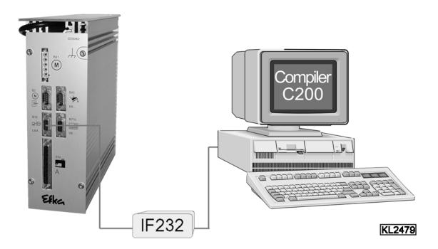
The control (socket B18) and the computer (socket com1) are connected by means of interface IF232-3.
