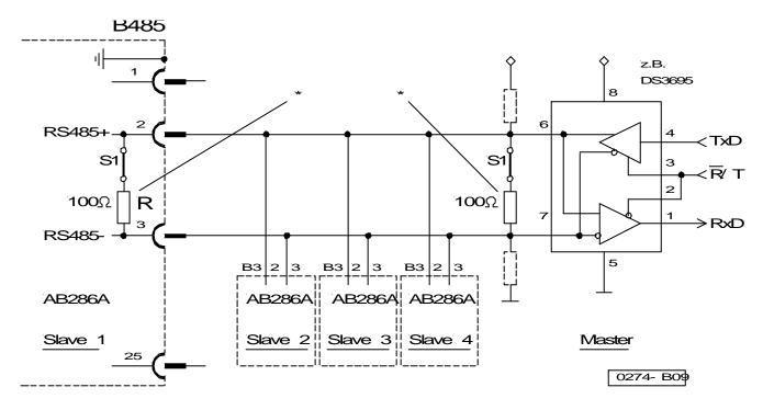
\* = Jumper S1 for terminating resistors
