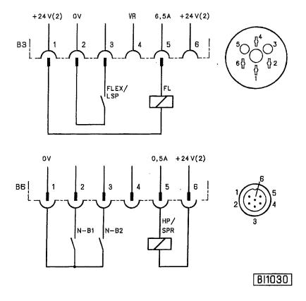
FL - Presser foot lifting HP - High lift walking
