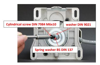
4.4 Use thooth belt to fix the thoothed belt wheel for tighten the cylindrical srew
