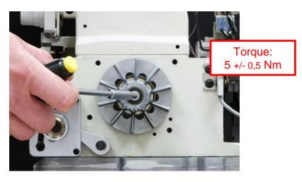
2.4 Fix the 2 headless screws in the toothed belt disc.
